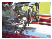
Single plate friction clutch for smooth pickup, precise control and easy engagement of the all-gear drive
