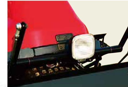
The headlight options are mounted on the front and rear. These lights are useful for early morning operation.
