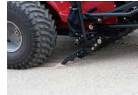
The cultivator option breaks up and softens coarse sand.
