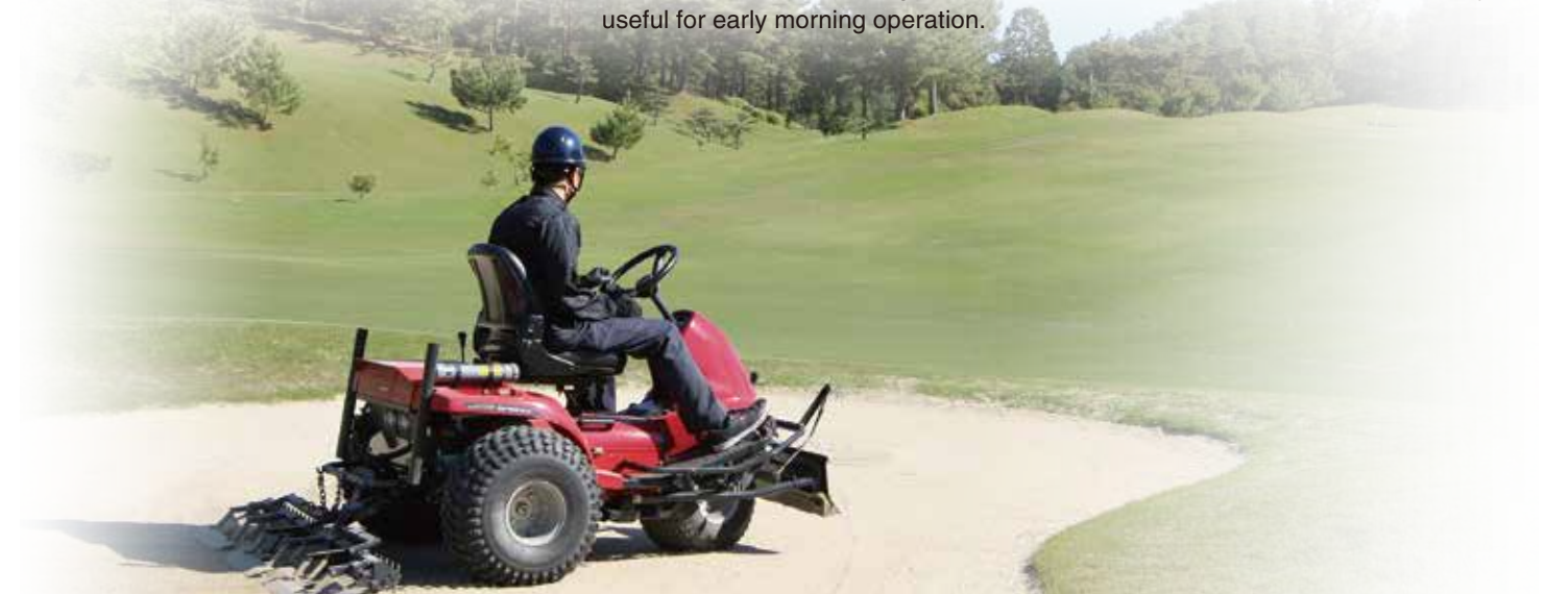
The cultivator option breaks up and softens coarse sand.
