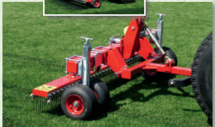
Optional the Verti-Groom can be equipped with 2 rows of Ø 3mm steel pins.
