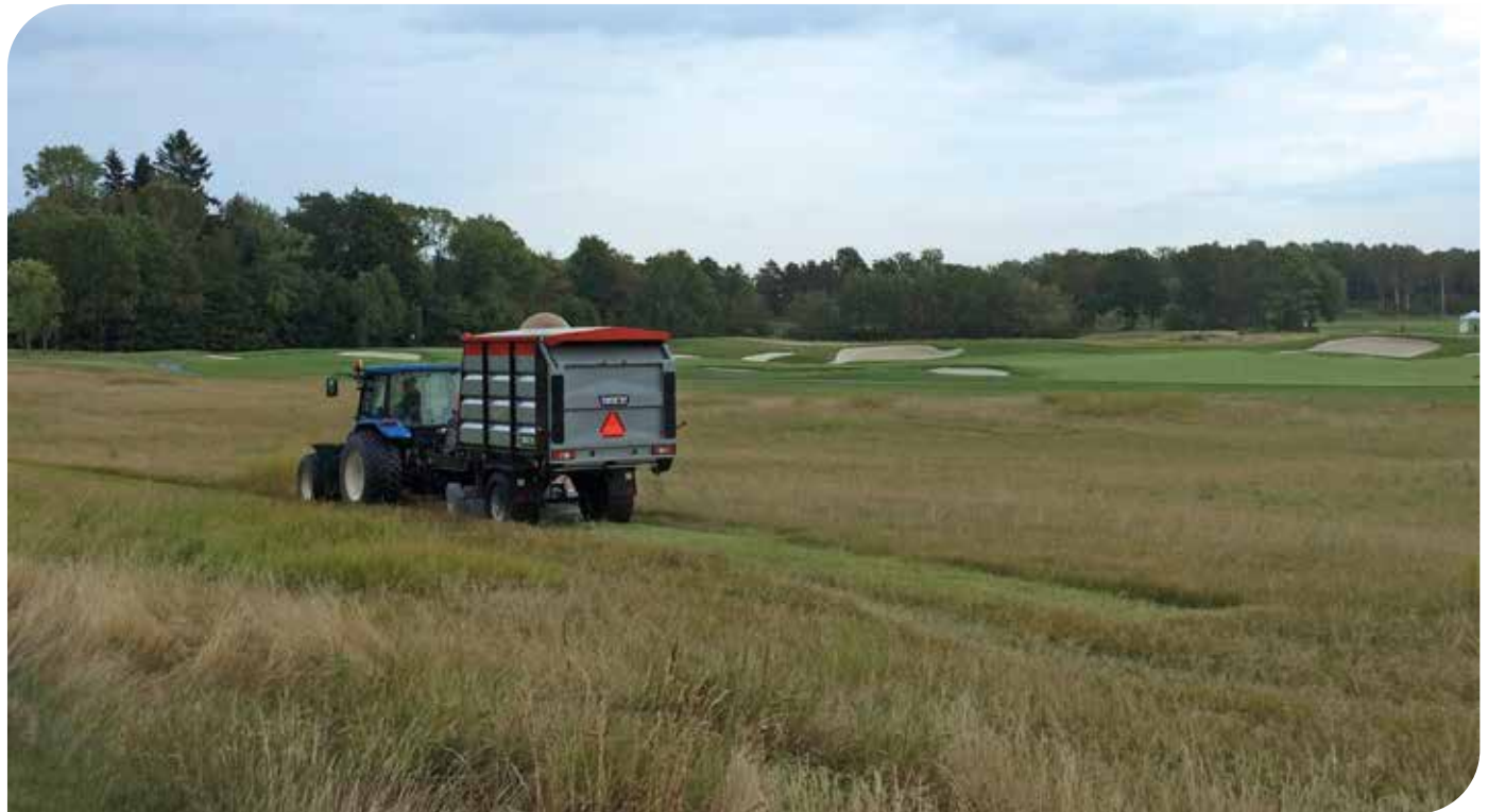
A TRILO C8 Large-size cut & collect vacuum sweeper mows and collects the rough in one pass.
