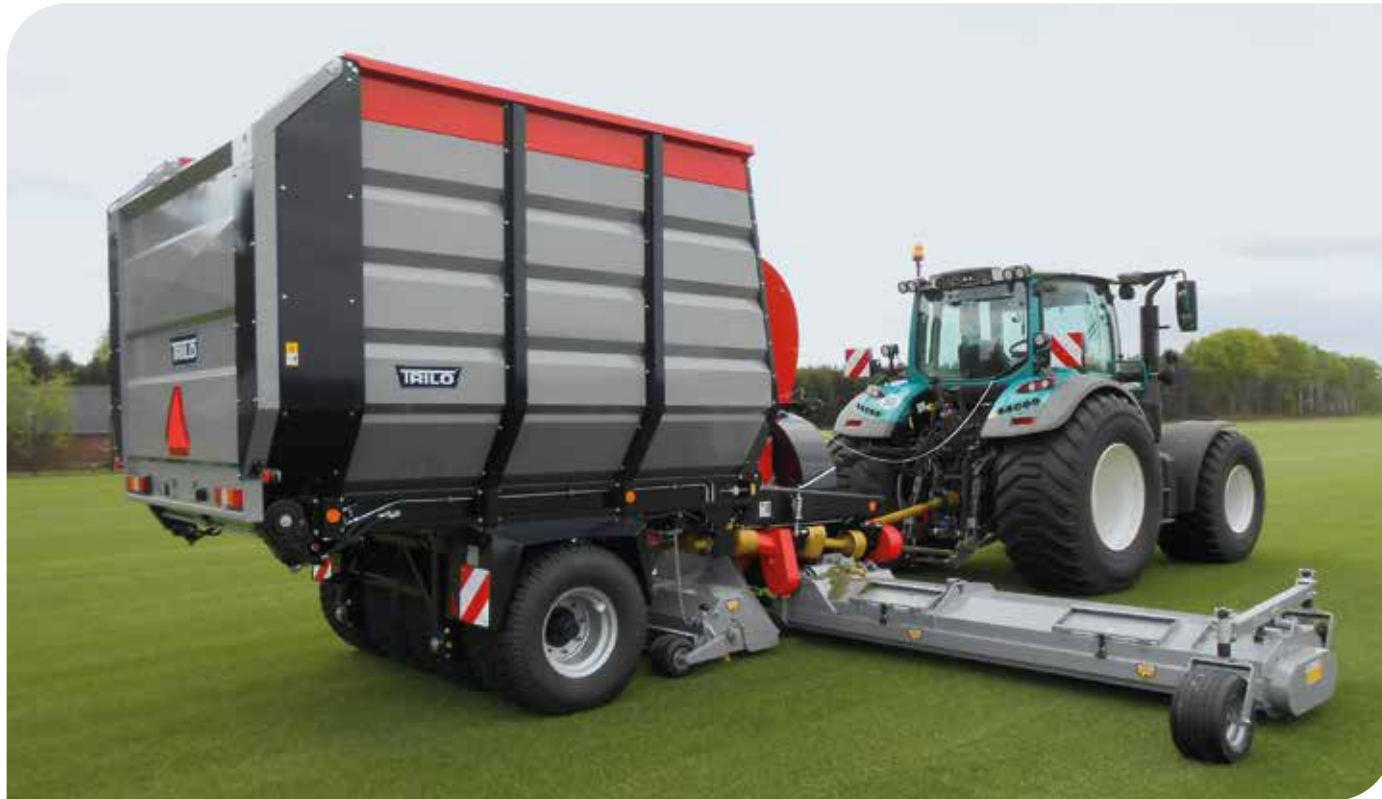
TRILO W (wide-area) Sweep & Collect vacuum sweepers with wings for sweeping and collecting large areas on golf courses.
